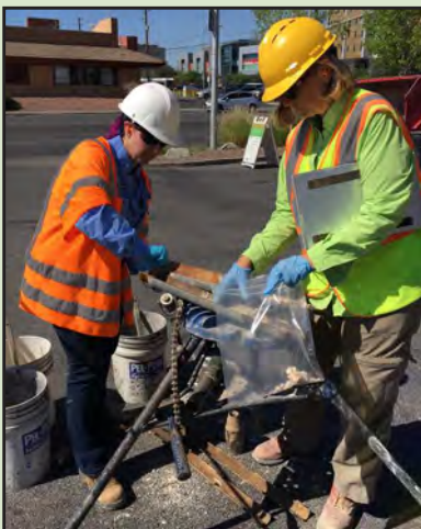
BEC scientists collecting soil samples from split spoon tubes. Source: BEC files.
