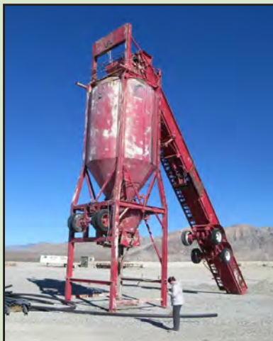
Red asphalt hopper observed in central portion of site. Source: BEC files.
